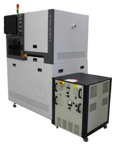
The **TF-3050 Series 3 LEP50** provides high accuracy performance to overcome the new challenges of smaller geometries of chip resistor trimming. Proprietary designs achieve the high accuracy mechanical positioning and ultra-stable laser beam control demanded by industry. **TF-3050 S3** utilizes vision registration theta rotation within a Windows XP operating system. These advance features are integrated with established substrate handling and automation systems.
